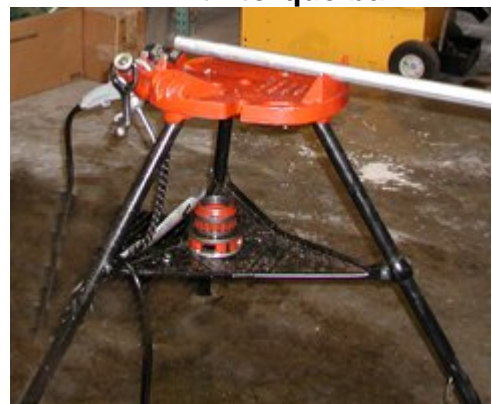
Figure 7 Vice mounted on a three-legged stand.
